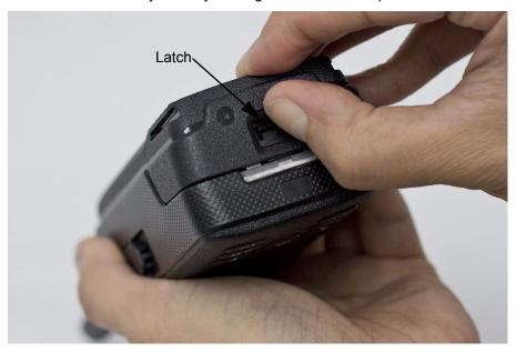
Figure 5-1. Battery removal
