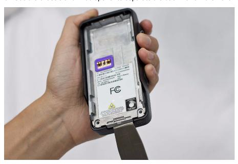
Figure 5-6. Back Kit disassembly
