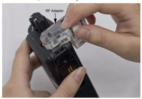
Figure 4-4. RF Adaptor insertion
