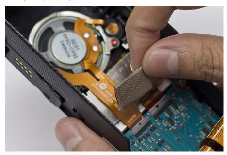
Figure 5-34. UC-Audio Flex Pad Reassembly
