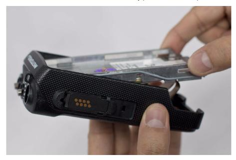
Figure 5-41. Front kit reassembly
