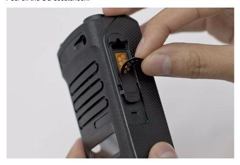
Figure 5-19. UC escutcheon removal.
