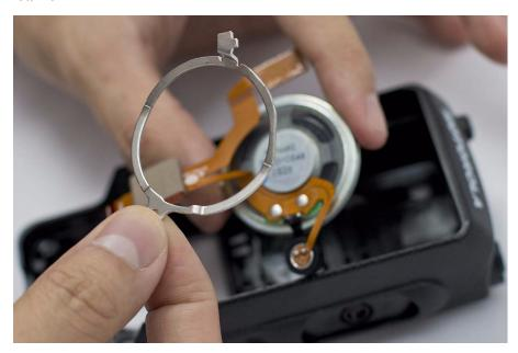
Figure 5-22. Speaker retainer removal
