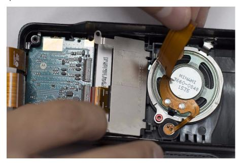
Figure 5-33. Speaker retainer reassembly
