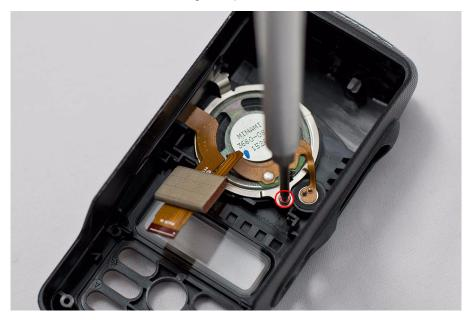
Figure 5-21. Speaker retainer screw removal
