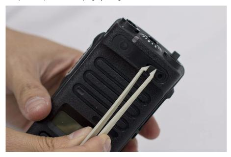
Figure 5-44. RF Plug reassembly
