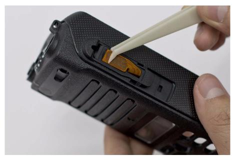
Figure 5-20. UC-audio flex removal
