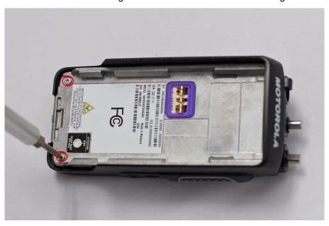
Figure 5-5. Front Kit-Back Kit Screw removal
