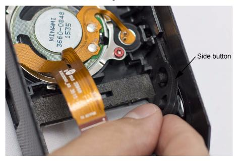
Figure 5-27. Side button reassembly
