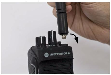
Figure 5-43. Attaching the antenna
