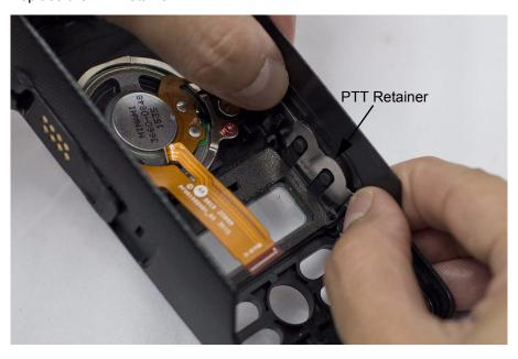
Figure 5-28. PTT retainer reassembly
