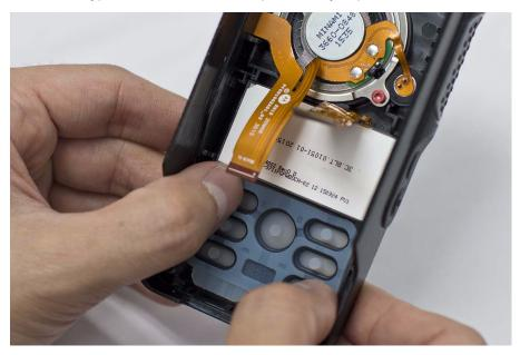
Figure 5-30. Keypad reassembly
