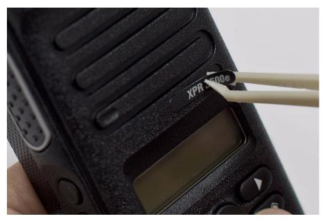
Figure 5-46. Product Nameplate Reassembly
