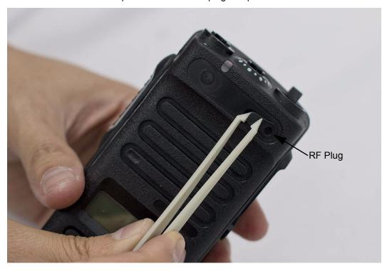
Figure 4-3. RF Plug disassembly
