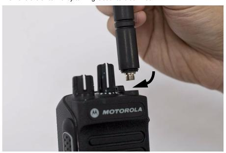
Figure 5-3. Antenna removal
