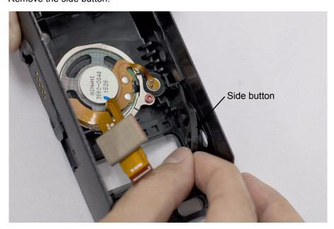
Figure 5-18. Side button removal
