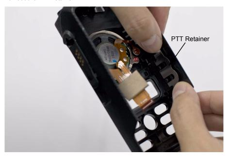
Figure 5-17. PTT retainer removal
