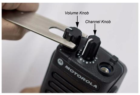
Figure 5-4. Volume and Channel Knob removal.
