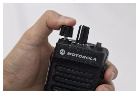
Figure 5-42. Knob reassembly
