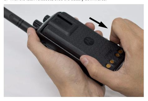
Figure 5-2. Battery removal
