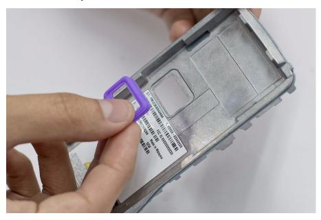
Figure 5-12. Battery contact seal removal
